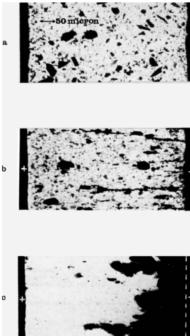
Fig. 1. Photomicrographs from thin cell arrangement (magnification 250X) of particles in 3:1 SRC filter feed. (a). No electric field. (b). 3 s after application of 100 V DC, and (c) 15 min after voltage applied.
